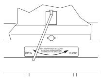
Figure 38 - Opening Vent Damper
